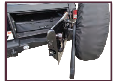
Rear Gate and Tire Carrier joined together to work in unison.
