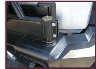
Adjustable, easy swivel hinge with grease fitting.
