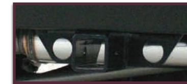
Bolt-On Receiver Hitch Included
