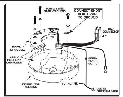
Figure 1 Installing the Module.
