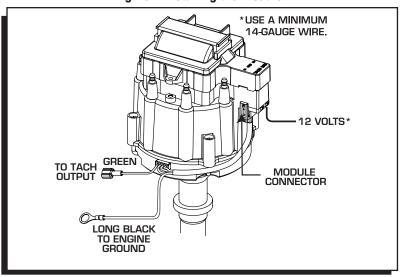
Figure 2 Connecting the Module and Tach Lead.
